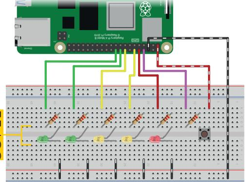
**Ensure your LEDs are inserted** the correct way around or they will not light-up. Long leg: anode (positive) Short leg: cathode (negative)
